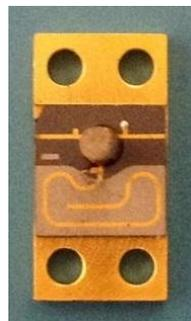
To protect the space communication payload electronics, Renaissance has designed a 26.5 GHz microstrip. Main features include compact size, low loss and high isolation. This device meets all of the NASA's outgassing requirements.
