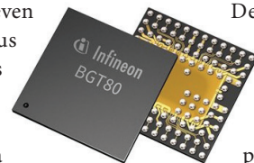
1. This E-band transceiver is intended for wireless-backhaul applications.
