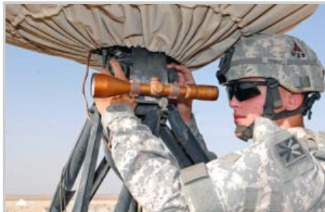
Calibrating the sights on a radar system in Iraq to constantly monitor the skies in search of indirect fire attacks. (Pfc. J. Princeville Lawrence)
