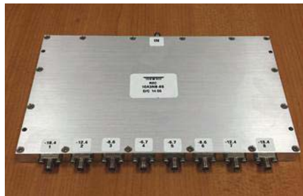
Model 10A3NB-8S is an eight-way power divider with tapered output levels for use in L-band systems from 1100 to 1500 MHz.
