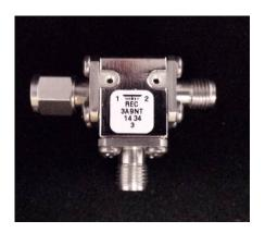
For high power Ku-band transceivers, Renaissance has developed a coaxial circulator operating between  $15-18\,\text{GHz}$  with 0.5 dB loss and 20 dB isolation in a compact size of 0.62" x .50" x .5".
