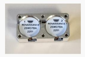
Designed to be used for Quantum Computing, this dual junction isolator operates at Cryogenic temperatures while providing low insertion loss and high isolation.
